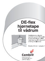
DE-flex corner tape made of synthetic rubber for sealing of corner joints wall-wall, wall-floor and pipe penetrations, Width 83 mm, length 10 m.
